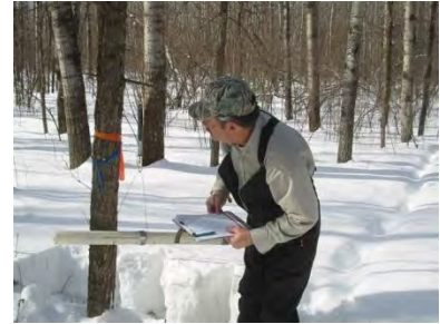
Establishing weight of snow sample to calculate water content
