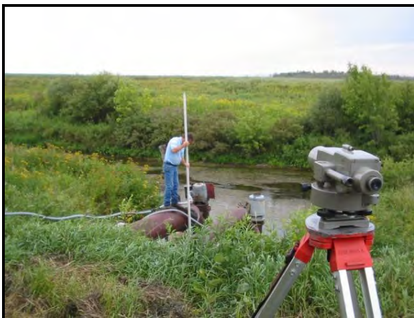
Surveying water lift from river to pump
