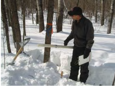
Establish base weight of empty sampling tube
