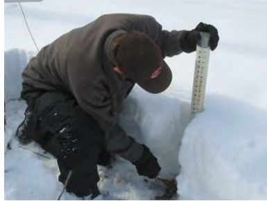
Obtaining snow depth and core sample
