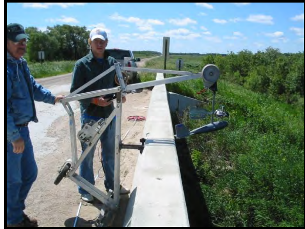
Measuring flow with bridge crane
