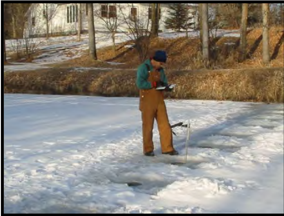
Measuring flow beneath ice
