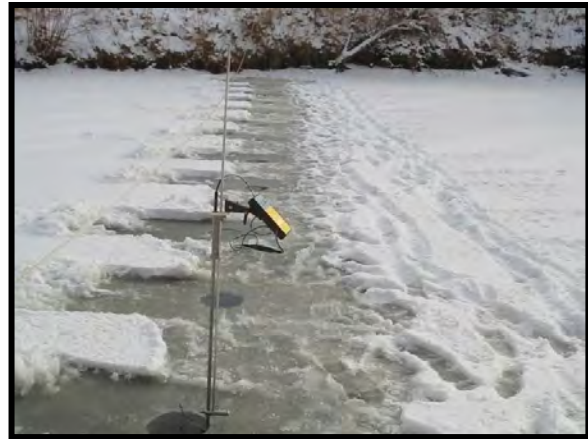
Measuring flow beneath ice
